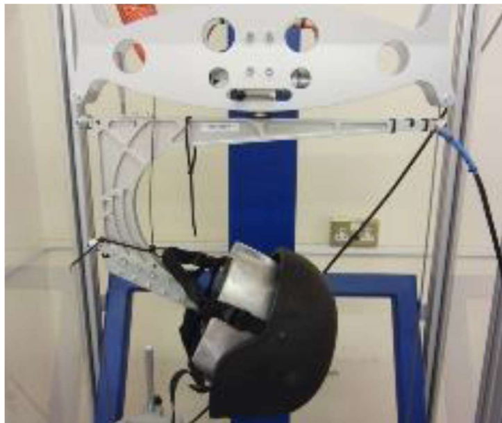
Figure 2 – Blunt impact protection testing setup
